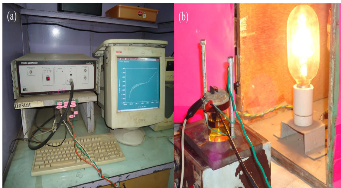
Fig. 5 (a) Experimental set up for ECPV cell performance study and (b) illuminated ECPV cell.
