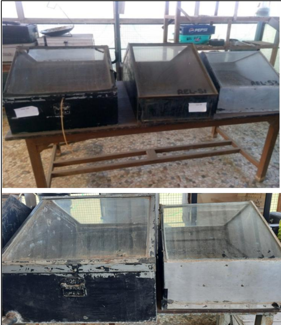
Fig. 5. Different types of Solar Stills
